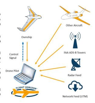
FlightHorizon GCS™ is designed to meet the FAA's Part 107.205 waiver requirements for beyond visual line-of-sight flights and the anticipated RTCA SC-228 Phase II Minimum Performance Standards.
