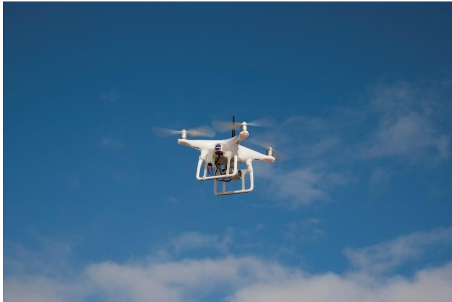
Fig. 6. Phantom 4 DJI Quadrotor Unmanned vehicle (NASA photo AFRC2016-0365-44).
