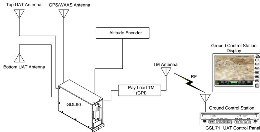
Fig. 1. ADS-B Out system architecture (Patent filed March 5, 2013; Serial No. 13/785,661).<sup>2</sup>
