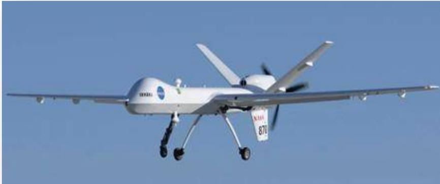
Fig. 4. Ikhana MQ-9 unmanned vehicle (NASA photo ED12-0082-22).
