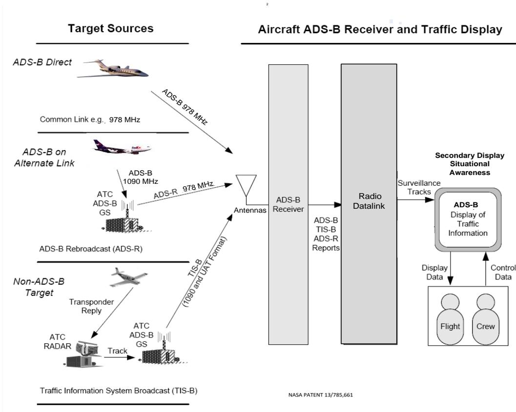
Fig. 2. ADS-B In system architecture (Patent filed March 5, 2013; Serial No. 13/785,661).<sup>2</sup>
